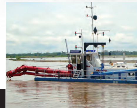
(Below) Cutter head suction dredge with SRR Dredge Suction hose
