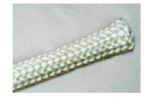
FUNCTION: Thermal Protection APPLICATION: Economical thermal protection over pipes, tubing, hoses, and cables in high-temperature environments. Extensively used in the oil and natural gas industries. Can be implemented under Pyrotex S/G sleeving for extra protection. Manufactured in both Heavy Wall (1/8" wall) and Light Wall (1/16" wall) varieties. COMPOSITION: Texturized E-Glass, braided CRITICAL TEMPERATURE: Continuous Exposure- 1000°F
