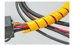
FUNCTION: Abrasion Protection APPLICATION: Spiral Guard Wrap provides protection and bundling for wire/cable assemblies wherever abrasion, cutting, or crushing is a potential hazard. Easily installed without the need to disconnect assemblies or uncouple hoses. Resistant to most oils, acids, and solvents. This material is flexible, reusable, and recyclable. COMPOSITION: High density polyethylene CRITICAL TEMPERATURE: -60°F to 200°F SIZES: 3/8″ ID – 5-1/2″ ID COLORS: Black, Yellow upon request
